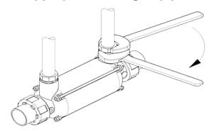
To prevent the stainless steel fitting from detaching itself from the heat exchanger housing and, as a result, also from the corrugated coil, and to prevent leaks from occurring, the stainless steel fitting should be firmly tightened with a second spanner or pliers.
